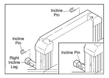
To change the incline, remove the incline pin from the right incline leg as shown.
